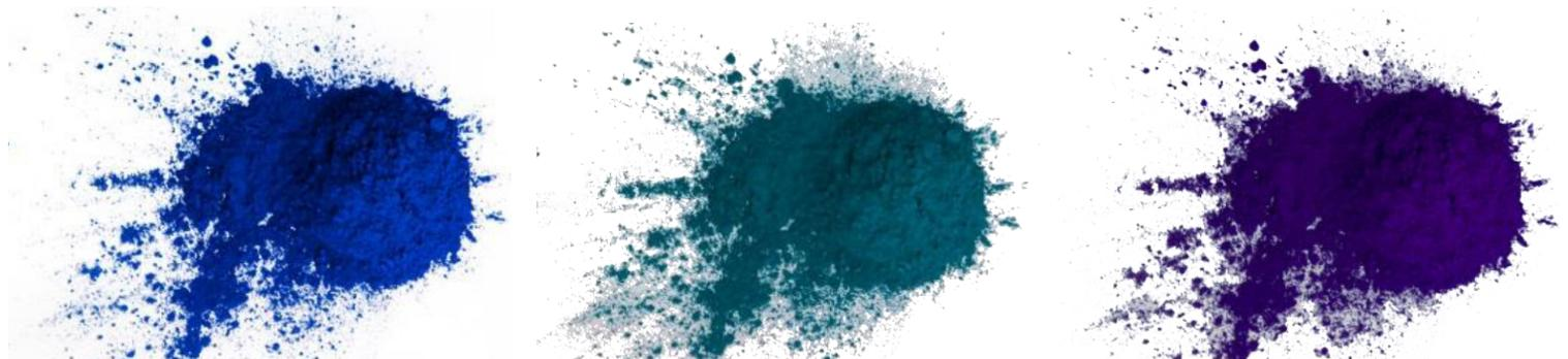
**Thin Wall Parts**– Poorly dispersed pigments in thin walls are a common cause of part rejection. Pre-colored polymers, especially those produced using twin screw compounding, provide substantially greater dispersion of pigments over masterbatches.
